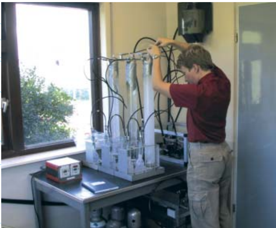
At the atmospheric monitoring station Lutjeward on the North Sea coast (The Netherlands), biweekly-integrated CO 2 samples are taken by absorption of CO 2 in sodium hydroxide
