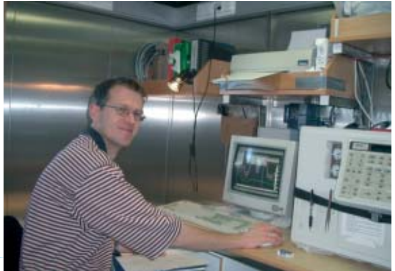
Anders Olsson determines freons in seawater by gaschromatography on board R/V G.O. Sars
