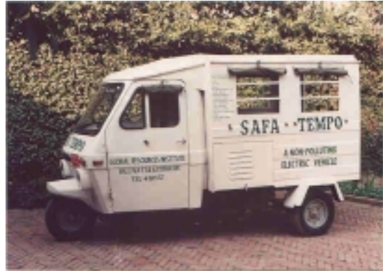
Figure B1. A typical battery operated three-wheeler in Kathmandu Valley (Courtesy: Clean Energy Nepal (CEN), Kathmandu, Nepal)
