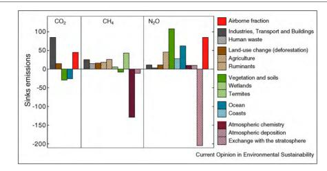
Emissions and sinks of CO<sub>2</sub>, CH<sub>4</sub> and N<sub>2</sub>O showing the interference of the human perturbations with the natural cycles. Numbers show the relative contribution (in percent) to the total emissions for each GHG. The fraction of the annual GHG emissions that stay in the atmosphere (the 'airborne fraction') is also shown in red. CO<sub>2</sub> figures are for 2000–2008 [3\*], CH<sub>4</sub> and N<sub>2</sub>O figures are for around 2000–2005 based on [17,18].
