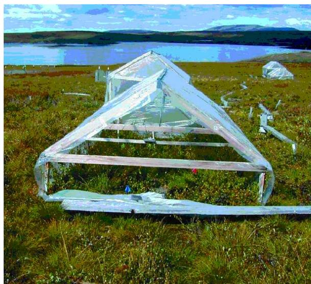
**Figure 5. The Toolik Lake Field Greenhouse Experiment in moist tussock tundra vegetation, Alaska, showing moderately increased abundance of deciduous shrubs and total vegetation mass. The photograph was taken in 1999, after 11 summers of warming. Photo: Gus Shaver.**
