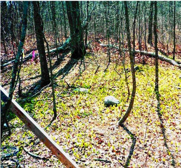
**Figure 4.** Harvard Forest Soil Warming Experiment, Massachusetts, showing early spring greening of forest floor. In this experiment, electric heating cables are buried 10 cm beneath the soil surface and 10 cm apart, along lines indicated by the string laid out on the surface. Photo: Kathy Newkirk.
